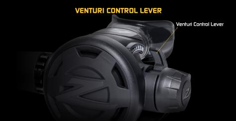
This lever controls the sensitivity of the regulator. The DIVE and PRE-DIVE Positions for the lever are marked on the case beside the lever. To avoid unexpected venturi free flows at the surface, or when entering into the water, the lever should be set in the PRE-DIVE (forward) position. As soon as the diver is ready to descend, the lever should be moved to the DIVE (back) position.
